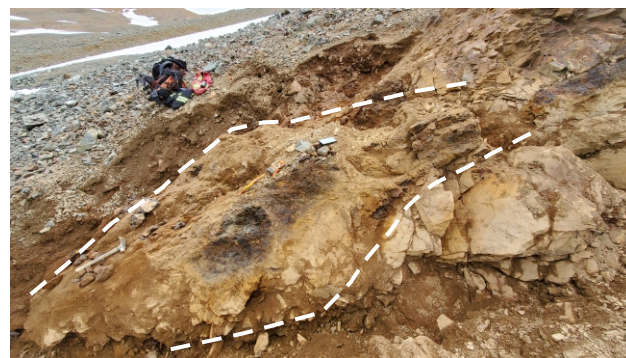
Semi-massive to massive sulphide lens (py, cpy) within altered basalt at the MS zone. A 2 m chip sample returned 1.3% Cu, 175 ppm Co and 4.5 g/t Ag.
