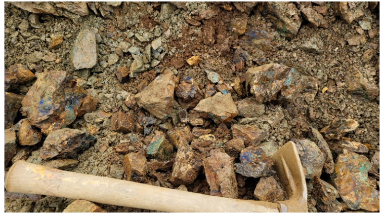
A portion of hand trench 22BATR004 that returned 1.18 g/t Au, 2088 ppm Co and 0.71% Cu over 5.7 m.
