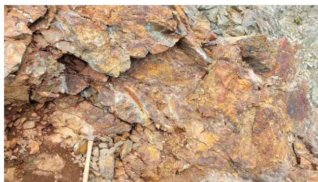
Quartz-sulphide breccia and stockwork in altered basalt. A 2 m chip sample through this zone returned 4.01 g/t Au, 0.51% Cu and 700 ppm Co.
