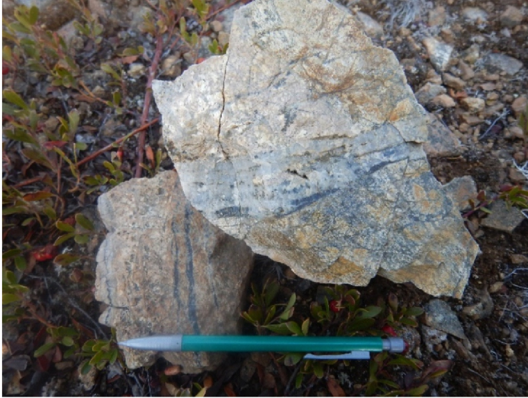
Quartz-biotite-magnetite veins developed within potassium feldspar altered porphyry from the core zone of the Maloney area.
